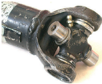
Figure 5.84 Detail of a universal joint
